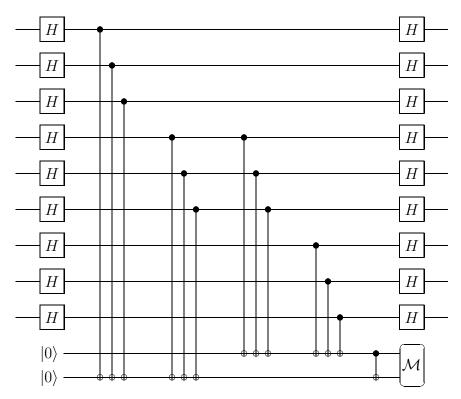
The measurement gives a syndrome that specifies, in binary, which of the three blocks has received a phase-flip error. Any phase-flip error can be corrected by applying a  $\sigma_z$  operation to **any one** of the three qubits in that block (or all three if you prefer).
