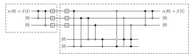
As you would expect, although the new code protects against phase-flips, it fails to protect against bit-flips (and in fact makes matters worse for bit-flips just as happened previously for phase-flips).
